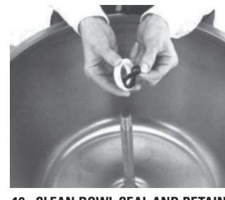
12. CLEAN BOWL SEAL AND RETAINER RING. Bowl seal and retainer ring easily snap on and off without tools. Wash if necessary, and dry. Replace and close cover.
