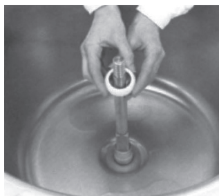
11. REMOVE BOWL SEAL AND RETAINER RING
